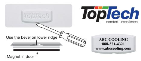
Gently slide a screwdriver into the bottom edge of the badge. Gently turn the screwdriver counter clockwise. The badge is held on by a magnet in the wall of the battery door. The badge should pry off easily. **Do not use force.**
