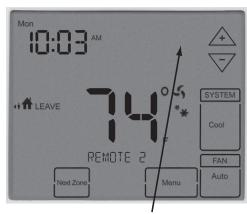
Setpoint will only be displayed for the zone currently being used by the program or in hold. Press the  $\triangle$  or  $\bigcirc$  to show the setpoint for adjustment.
