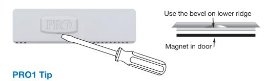
Gently slide a screwdriver into the bottom edge of the badge. Gently turn the screwdriver counter clockwise. The badge is held on by a magnet. The badge should pry off easily.
