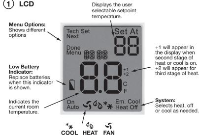
The **COOL**, **HEAT** or **FAN** icon will display when the **COOL**, **HEAT** or **FAN** is on.NOTE: The compressor delay feature is active if these icons are flashing. The compressor will not turn on until the 5 minute delay has elapsed.
