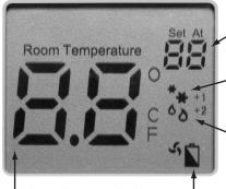
Low Battery Indicator: Replace batteries when indicator is shown.
